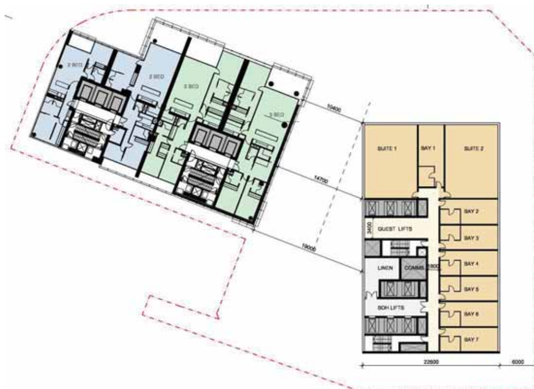
Figure 12: Revised building separation between towers, Levels 16 to 21 indicative floor plan (Source: Applicant's EIS)
